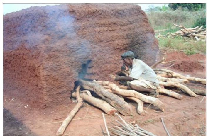
*Bricks being stacked up to an oven with 2 openings. After getting covered with much, fire is put inside and then sealed.*
